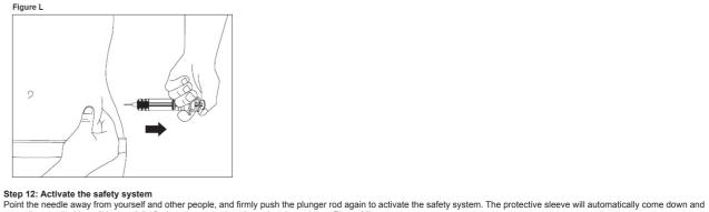
cover the needle. You will hear a "click" when the protective sleeve is released (see Figure M) You will feel some resistance. This is normal. Keep pushing until you hear the "click." The safety system can only be activated after the syringe has been emptied. Only activate the safety system after you have removed the needle from your skin.
